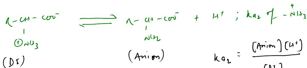
$$k_{a_2} = \frac{[\text{Anion}][\text{H}^+]}{[\text{DI}]} \Rightarrow [\text{Anion}] = \frac{k_{a_2} \cdot [\text{DI}]}{[\text{H}^+]} \quad \text{--- (2)}$$
