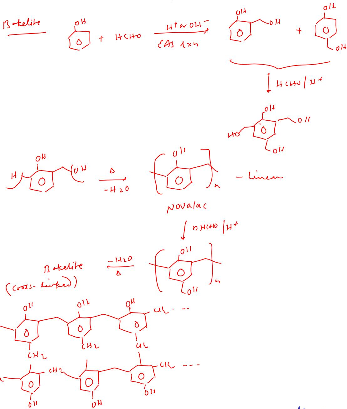
Bakelite is used as molding combs, phonograph records, electrical switches and handles of various utensils.
