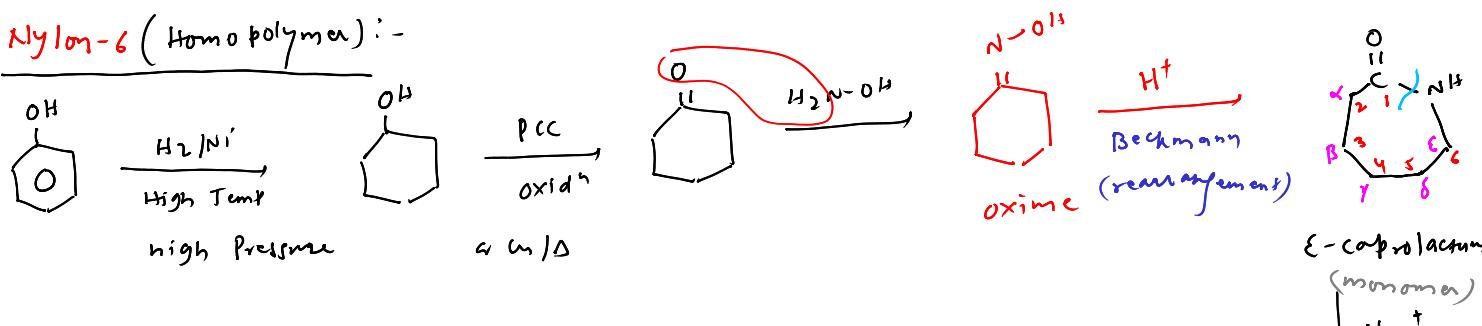
Nylon-6 is used in making tyre cords, fabric and ropes
