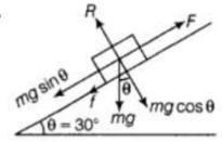
Mass of the block m = 1 kg Angle of inclination =  $30^{\circ}$ Coefficient of friction = 0.1 Displacement = 10 m
