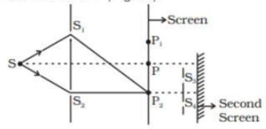
At P<sub>2</sub> on the screen, there is a hole and behind P<sub>2</sub> is a second 2- slit arrangement with slits S<sub>3</sub>, S<sub>4</sub> and a second screen behind them.
