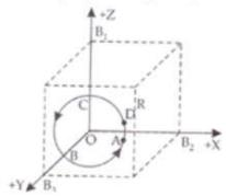
So Magnetic field due to quadrants AB, BC, and CD at their centre O are B<sub>1</sub>, B<sub>2</sub>, and B<sub>3</sub> respectively is given below:-
