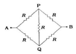
It is a balanced Wheatstone bridge. Hence, resistance in the branch PQ can be removed without affecting the effective resistance of the circuit. Hence, the
