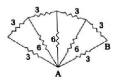
Sol. In the leftmost loop, two  $3\Omega$  resistors are connected in parallel to one  $6\Omega$  resistor. Effective resistance of this loop is  $R = (3+3) \parallel 6 = 6 \parallel 6 = 3\Omega$ .
