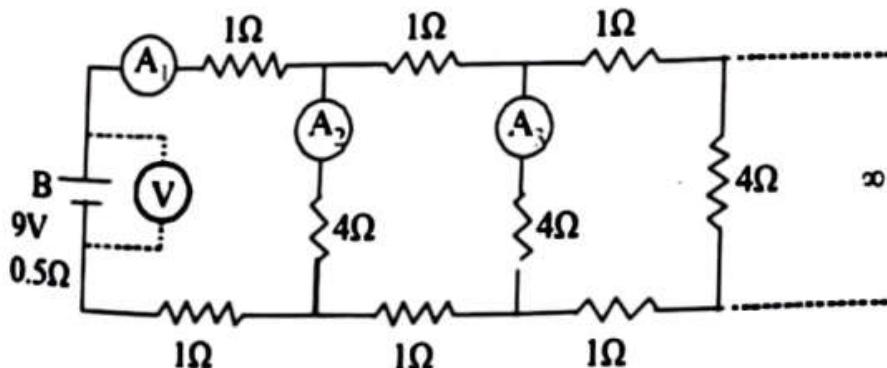
A 9 V battery with internal resistance of  $0.5 \Omega$  is connected across an infinite network as shown in the figure. All ammeters  $A_1$ ,  $A_2$ ,  $A_3$  and voltmeter  $V$  are ideal.
