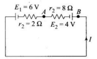
**Solution:** Key concept: In this problem, after finding the electric current flow in the circuit by using Kirchoff's law or Ohm's law, the potential difference across AB can be obtained.
