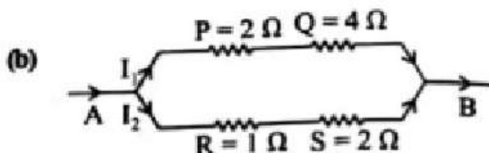
$$R_1 = P + Q = 2\Omega + 4\Omega = 6\Omega$$
