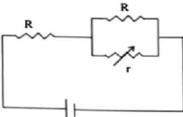
In the circuit shown, the resistance  $r$  is a variable resistance. If for  $r = fR$ , the heat generation in  $r$  is maximum then the value of  $f$  is : [Online April 9, 2016]
