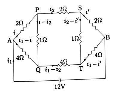
We claim, by symmetry, that i = i' because circuit looks symmetrical when we see it from either node A or B. This can be shown by applying Kirchhoff's loop law in loops APQA and SBTS which gives
