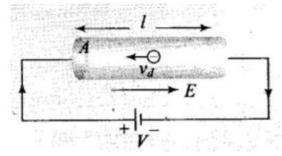
The direction of drift velocity for electron in a metal is opposite to that of applied electric field (i.e. current density  $\vec{J}$ ).
