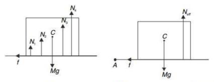
(b) About the centre (C) of the block there is no rotation. Mg has no torque about C. Friction has a clockwise torque
