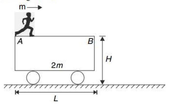
Let displacement of the cart be  $x \leftarrow b$  by the time man reaches the edge B. Since centre of mass of the system (Man + Cart) will remain at rest hence,
