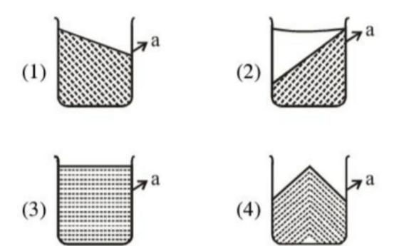
Diagram (1) represents surface of liquid when the container is sujected to acceleration .
