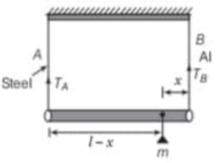
Let T<sub>A</sub> and T<sub>B</sub> be the tensions in wire A and wire B respectively. For the rotational equilibrium of the system,
