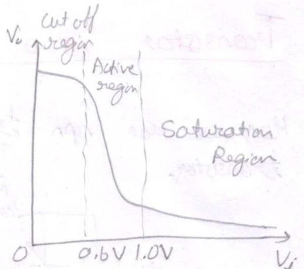
if  $V_i$  is high ( $V_i > 1.0\text{ V}$ ),  $V_o$  is low  $\approx 0$
