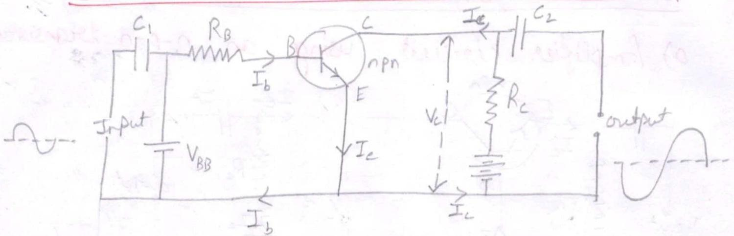
Input circuit is forward biased & output is reversed.
