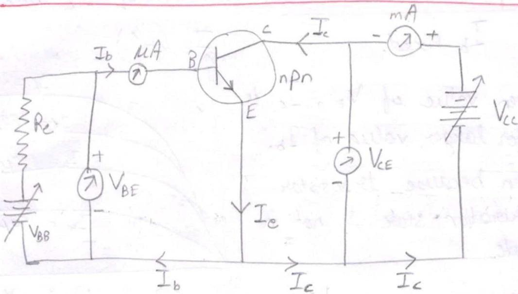
Input characteristics: Relation between  $I_b \rightarrow V_{BE}$
