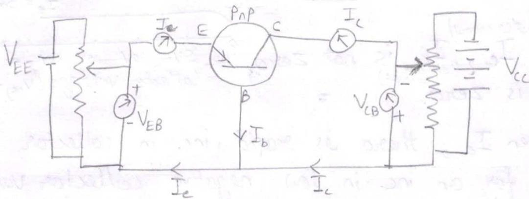
→ Emitter base circuit is forward biased with  $V_{EE}$
