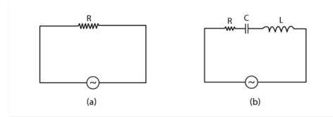
(a) Under which conditions would the rms currents in the two circuits be the same? (b) Can the rms current in the circuit (b) be larger than that in (a)?
