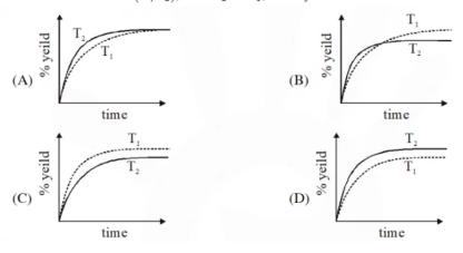
Sol. (B) At t = 0  $\Rightarrow$   $r_{net} = k_f [N_2][H_2]^3 = r_f$ . % yield will increase in initial stages due to increase in net speedAs time proceeds  $\Rightarrow$   $r_{net} = k_f [N_2][H_2]^3 - k_b [NH_3]^2$ On increasing temp.,  $k_f \& k_b$  increasebut increase of  $k_b$  is moreso % yield will decrease% yield will increase in initial stage due to enhance speed but as time proceeds, final yield is governed by thermodynamics due to which yield decrease since reaction is exothermic
