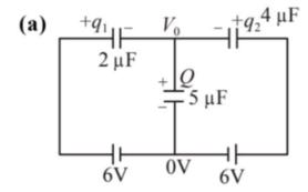
Let  $q_1$  and  $q_2$  be the charge on the capacitors of  $2\mu F$  and  $4\mu F$ . Then charge on capacitor of  $5\mu F$
