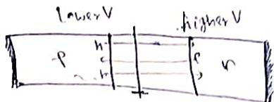
$I_{\text{diffusion}}$  :- Majority carriers try to diffuse on the other side because of concentration gradient and facing the opposition of this depletion layer electric field still some are able to cross and that creates Diffusion current from p to n.
