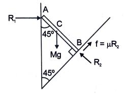
Balacing torque about point A,  $f\ell = Mg\left(\frac{\ell}{2}\sin 45^\circ\right)$
