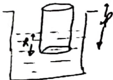
$\sigma$  = density of cylinder $\rho$  = density of fluid ( $\sigma > \rho$ )
