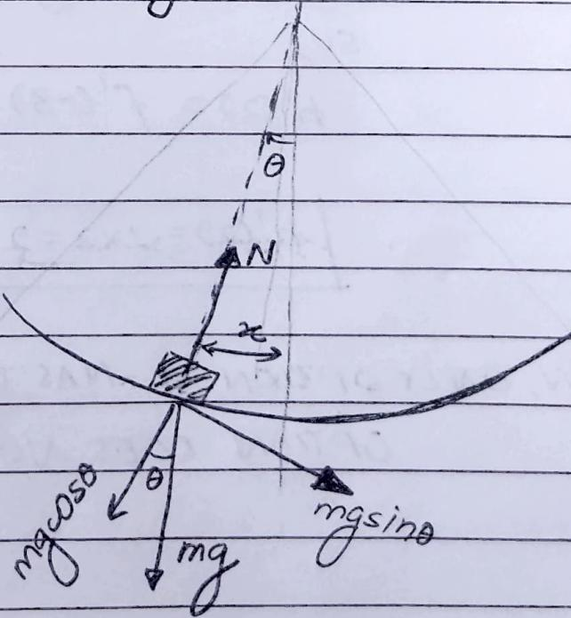
$$\text{So, } -ma = mg \frac{x}{R} \Rightarrow a = -\frac{g}{R} x \text{ which follows SHM}$$
