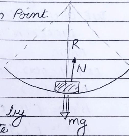
Step 2: Displace the mass by 'x' and then calculate restoring force to find the acceleration (restoring)
