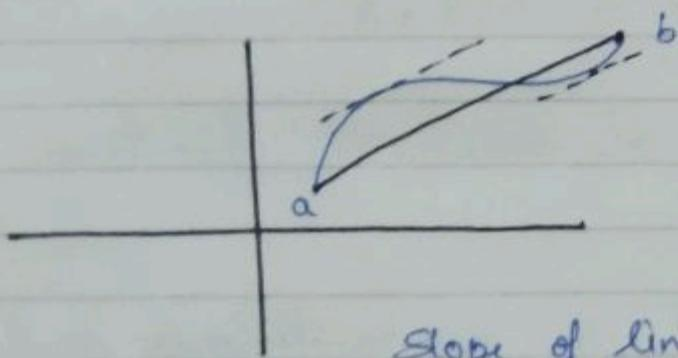
Slope of line joining  ~~$(a, f(a))$  and  $(b, f(b))$~~  is  $\frac{f(b) - f(a)}{b - a}$
