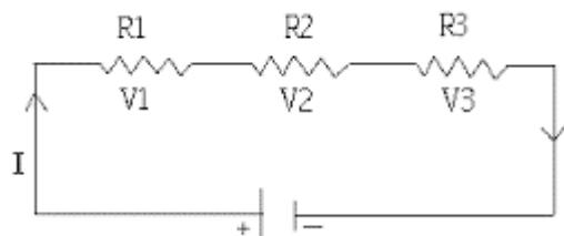
**Kirchhoff's voltage law:-**  $V_1 + V_2 + V_3$
