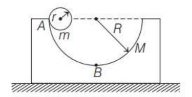
(a) The centre of mass of M + m in this case will not move in horizontal direction. Let M moves towards left by a distance x then m will move towards right by a distance R - r - x (with respect to ground). For centre of mass not to move along horizontal we should have
