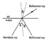
Also, the Snell's law  $\mu_1 \sin \theta_1 = \mu_2 \sin \theta_2$  tells that the angle of refraction will be more than the angle of incidence, on entering the air the ray will bend away from the normal. See the diagram.
