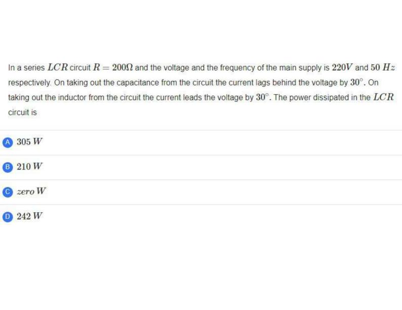
4. In given LCR circuit, R = 200 S and Vrand = 220V, V = 50 HZ = W= 2RV = Lours 1001 rad/) When capacitor is taken out, then it becomes L-R:-= tand = X1 (d=30 given) = tau3i = X, 7 X = 200 S When inductor is taken out, then it becomes R-C circuits : tand = x (\$ = 30 given) 7 tau30 = Xc => Xc = 200 sc NOW, X = - X = 2w - 2w => 0 55 55 : 2 = JR2+ (xc-x,)2  $=5(200)^2 + 0$ =7 [2 = 200 52]
