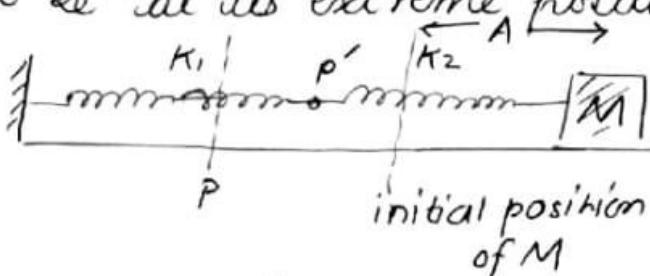
\* Now both the springs would stretch to compensate for this amplitude 'A'. i.e  $\boxed{\text{stretch}_1 + \text{stretch}_2 = A}$
