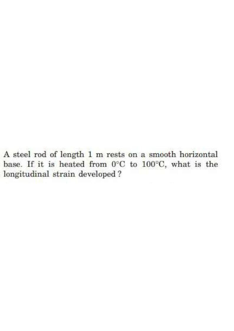
Steel rod is resting on a smooth horizontal bake at 0°C. When temperature is increased to lov'C, it will lead to an increase in the length of steel due to expansion on heating. But, because there is no opposition in expansion of length, no longitudinal strain will be developed.
